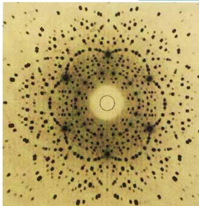
(top) The pattern produced by electron diffraction of a titanium/nickel alloy. (bottom) Pattern produced by X-ray diffraction of a beryl crystal.
