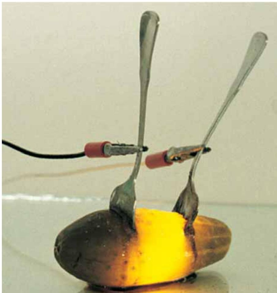
When alternating current at 110 volts is applied to a dill pickle, a glowing discharge occurs. The current flowing between the electrodes (forks), which is supported by the  $\text{Na}^+$  and  $\text{Cl}^-$  ions present, apparently cause some sodium atoms to form in an excited state. When these atoms relax to the ground state, they emit visible light at 589 nm, producing the yellow glow reminiscent of sodium vapor lamps.
