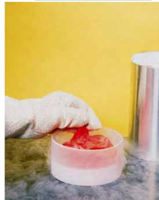
(a) A balloon filled with air at room temperature. (b) The balloon is dipped into liquid nitrogen at 77 K. (c) The balloon collapses as the molecules inside slow down due to the decreased temperature. Slower molecules produce a lower pressure.
