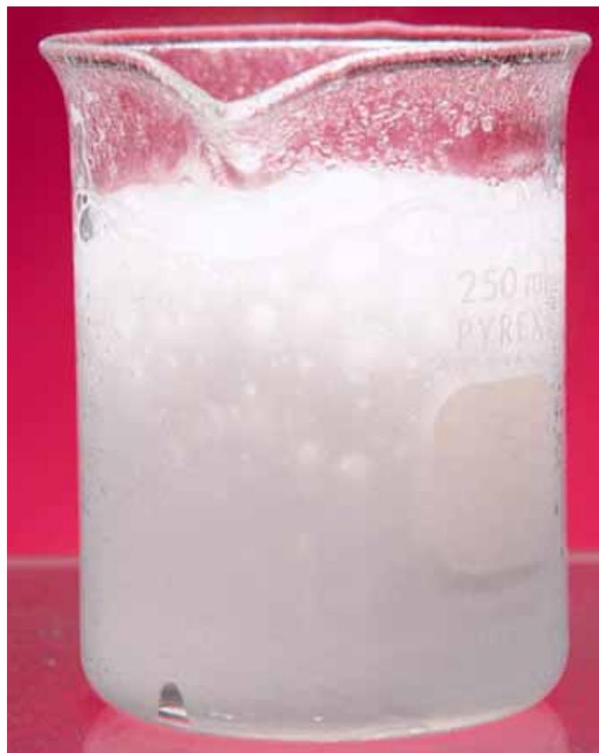
Hydrochloric acid reacts with solid sodium hydrogen carbonate to produce gaseous carbon dioxide.
