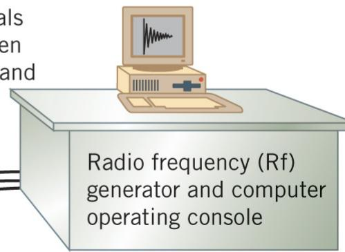
Fourier transformation of the signal from the time domain to the frequency domain occurs at the computer console.
